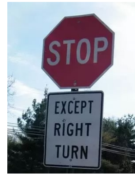
Figure 6 Recommended sign configuration.
