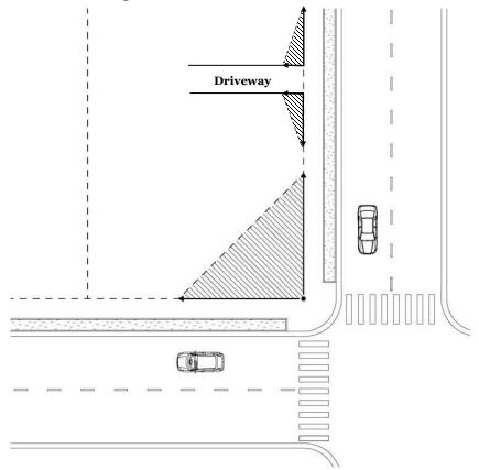
• The area in a Vision Triangle shall be kept unobstructed from 2.5 ft to 10 ft above the elevation of the centerline of the intersection, except for traffic signs, public utility poles, single-stem tree trunks and similar features.
