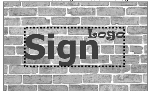
Exhibit 4. Measuring the area of a wall sign
