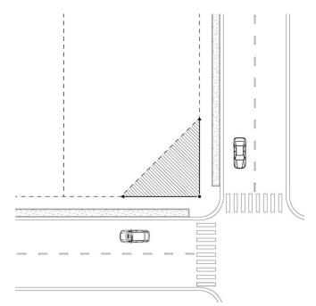
• The area in a Vision Triangle shall be kept unobstructed from 2.5 ft to 10 ft above the elevation of the centerline of the intersection, except for traffic signs, public utility poles, single-stem tree trunks and similar features.
